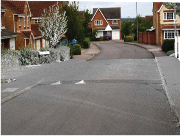
By extracting colours from oblique mobile images to laser points, 3D-views are photo-realistic what ever you are looking at.
