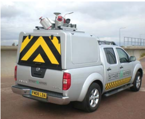
In a typical mobile Lidar system scanners, cameras and IMU/GPS are mounted on vehicle roof.
